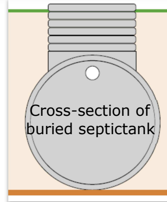
Septictank - Model KWH WehoSeptic, 2500 l.
